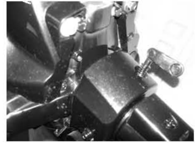
1. Cooling water checking hole
