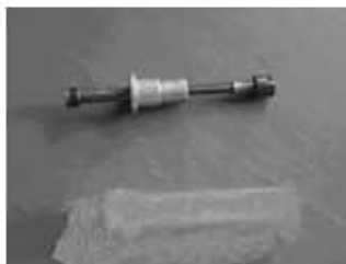
Sleeve bearing with guard board installer tool
